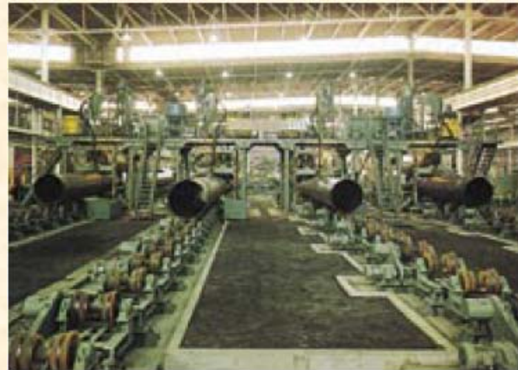
Automatic outside submerged arc welders
